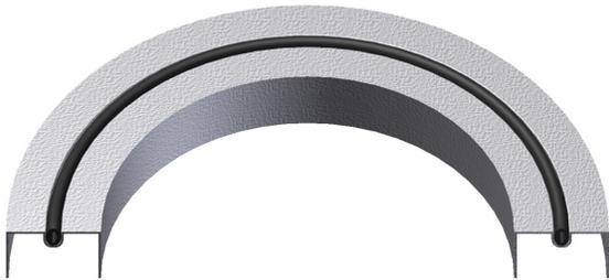
Cross section of a stamped groove
