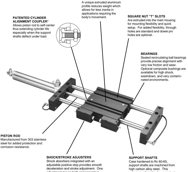
adjustable positive stop provides smooth deceleration and stroke adjustment. One adjustment moves both components in unison – eliminating multiple iterations during setup. Shocks can be added in the field. Case hardened to Rc 60-65, support shafts are machined from high carbon alloy steel. This extreme surface hardness protects the shaft's round ways from nicks and scratches - enhancing component life and reducing maintenance.
