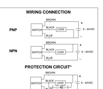
\* When connecting an inductive load (relay, solenoid valve, etc.), a protection circuit is recommended. Use a 100V, 1A diode. (NPN connection shown.)
