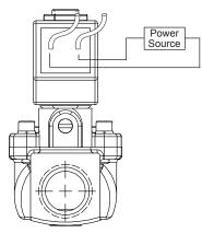
Flving Leads Power leads connected to coil flying leads. No earth around present.
