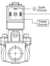
**DIN Connector** Power leads connected to vertical pins on all versions. Horizontal pin is earth ground on all versions.
