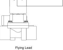
Flying Lead Power leads connected to coil flying leads. No earth ground present.
