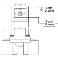
DIN Connector Power leads connected to verticle pins on all versions. Horizontal pin is earth ground on all versions.
