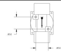
Mount on pipe in any position or #10-32 machine screws in base.
