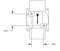
Mount on pipe in any position or #10-32 machine screws in base.
