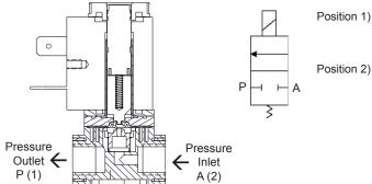
Position 1) Coil De-energized. Pressure inlet port A (2) is closed from outlet port P(1).
