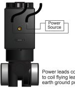
Power leads connected to coil flying leads. No earth ground present.
