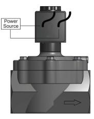
Flying Lead Power leads connected to coil flying leads. No earth ground present.
