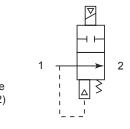
Position 1) Coil de-energized. Pressure inlet
