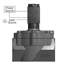
**DIN Connector** Power leads connected to verticle pins on all versions. Horizontal pin is earth ground on all versions.
