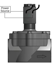
Flying Lead Power leads connected to coil flying leads. No earth ground present.
