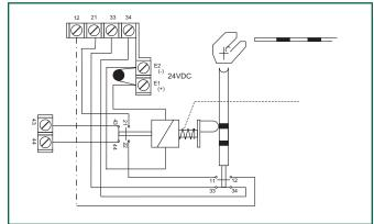
\* Actuating key not inserted and solenoid unlocked.
