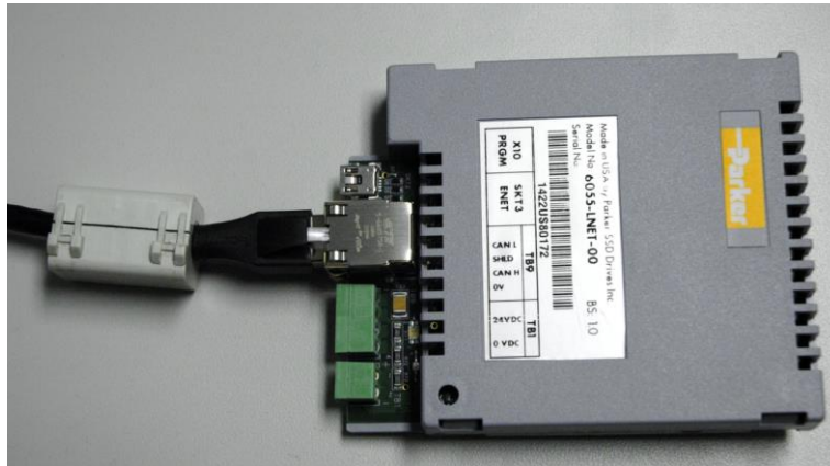
6055-LNET-00 TECHBOX with FERRITE CORE Installed
