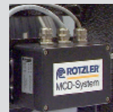
Measuring control device (MCD)
