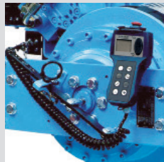
Operating unit (wired remote control) to ensure winch control
