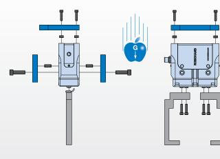
Body mounts with screws and locates with slip fit dowel pins for accuracy Fingers attach to jaws with screws and locate with dowel pins
