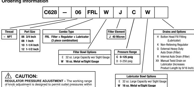
of knob adjustment is designed to permit outlet pressures within their full range. Pressure adjustment beyond this range is also possible because the knob is not a limiting device. This is a common characteristic of most industrial regulators, and limiting devices may be obtained only by special design.
