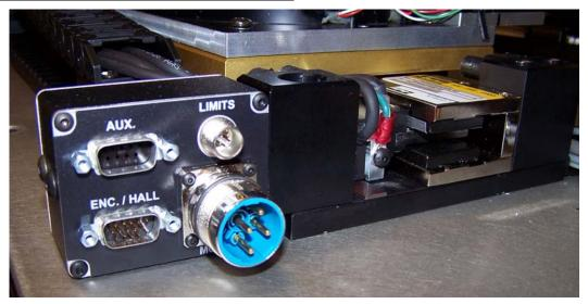
Trilogy positioners have a connector box option as a standard option. Daedal LXR users will recognize this as similar to the LXR connector box. This is allows users to be able to quickly connect Trilogy positioners to standard Parker drives with pre-connectorized cables. The connector box is available with Flying leads or Parker-drive connectorized cables in 3 or 7.5 meter (10 or 25-foot) for Aries, Compax3, Gemini or ViX servo drive/controllers.
