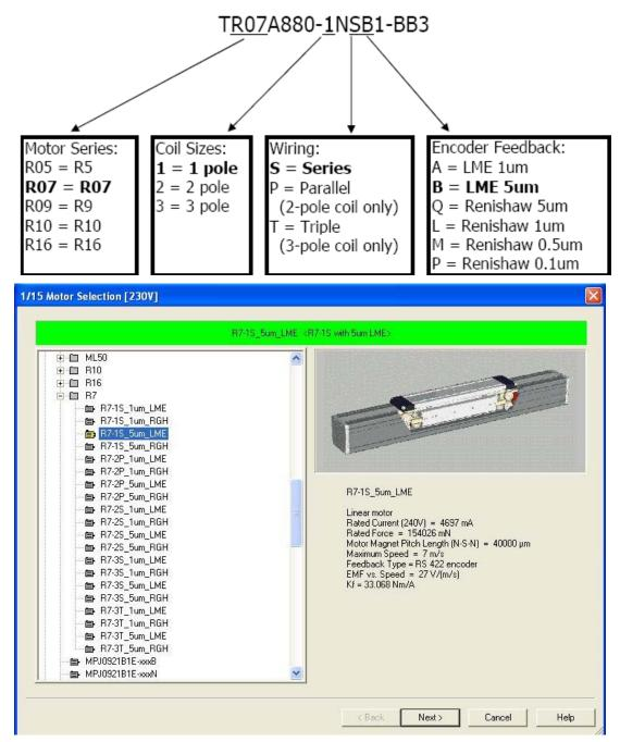
Note that the Compax3's motor database should be updated. The file is available for download at: <a href="http://www.compumotor.com/bbs/FAQ/CPX3">http://www.compumotor.com/bbs/FAQ/CPX3</a> USMOTOR rev14.zip
