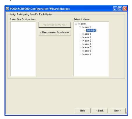
The Masters screen allows the Axis to be attached is the Master, which is the motion trajectory calculator.
