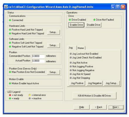
This screen allows enabling the axis, simple jogging and can verify limit switch functionality. Note that the maximum position error is set to 1, whether that is 1mm or 1inch; set appropriately.
