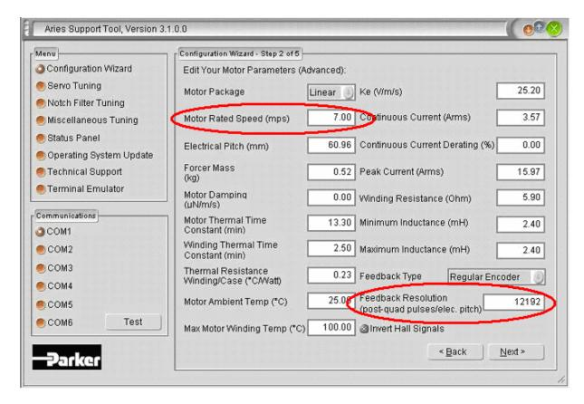
The R7-1 with 5um magnetic would be set to 8000 counts/electrical pitch. Note that the halls are inverted for both I-Force and Ripped series coils for Aries configuration.
