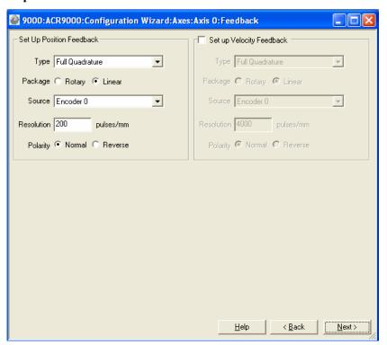
For feedback resolution for the ACR9000, select normal polarity and set the resolution. Standard resolution settings are listed in the following table:
