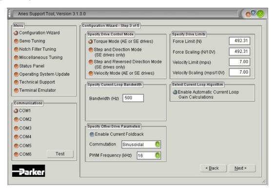
When using the Aries with an ACR9000, in step 3 of 5 of the AST's Configuration Wizard set the drive in torque mode. Set the current loop bandwidth to 500Hz. This can be increased in current loop tuning if necessary. As the drive is in torque mode the velocity limit in this screen is not used.
