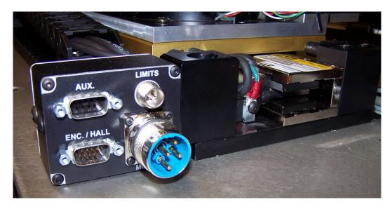
Trilogy positioners have a connector box option as a standard option. Daedal LXR users will recognize this as similar to the LXR connector box. This allows users to be able to quickly connect Trilogy positioners to standard Parker drives with connectorized cables. The connector box is available with Flying leads or Parker-drive connectorized cables in 3 or 7.5 meter (10 or 25-foot) for Aries, Compax3, Gemini or ViX servo drive/controllers.
