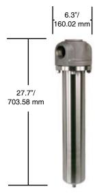
**Application: Finite**'s 2" NPT stainless steel filter is the right solution for most critical or corrosive compressed air/gas applications. Its 500 PSIG design pressure makes this an ideal choice for higher pressure applications. Bulk liquid separating, coalescing, particulate and adsorptive filters are available. Includes 1/4" NPT drain port with plug.
