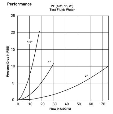
The Parker PF Series Dry Disconnect couplings virtually eliminate fluid loss upon disconnection and are designed help meet the demand for closed system transfer and dispensing of chemicals and fluids with minimal environmental contamination. They can be used with concentrated or diluted industrial chemicals, fertilizers, herbicides, insecticides, fungicides or pesticides when transferring from bulk storage tanks, returnable containers, applicators, etc.
