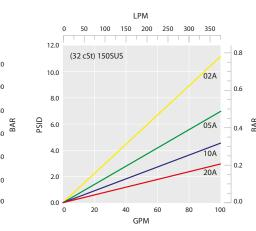
Correct for other fluids by multiplying new viscosity in cSt/32 (SUS/150) x new S.g./0.9
