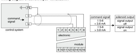
The 4...20mA option uses the "0mA" condition as breakdown-information. This means the presence of an evaluable failure information if the input signal line is interrupted. In this case the solenoid output will be switched off. The output will switched on when the input signal reaches a value of 3.8mA, it switches
