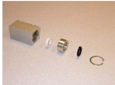
Photo 1B: Carriage seal replacement
