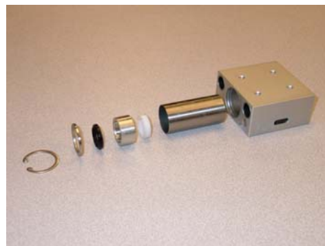
Photo #2B: Carriage seal replacement
