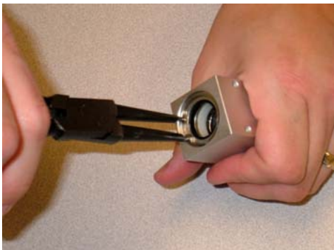
Photo 1A: Snap Ring removal
