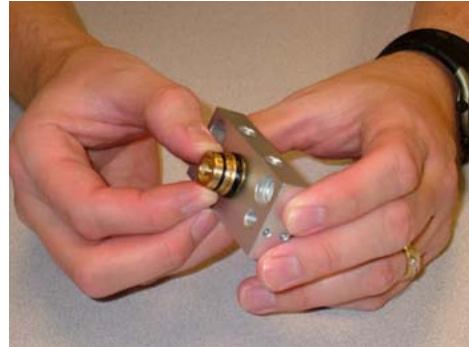
Photo #1: Pilot Insert O-rings
