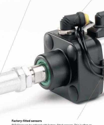
P1D Clean can be ordered with factory-fitted sensors. This is often an advantage for other cylinder versions as well. These cylinders come with the sensors mounted in the end positions. If needed, the sensors are easy to adjust when installing the cylinders. Choose from a wide range of sensors – electronic or reed type, 3 or 10 metres of cable, 8 mm or M12 connectors.
