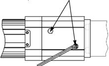
• Insert the plugs into the coupling housing to prevent the penetration of dirt.
