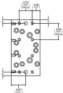
OAI = BASE LENGTH + 1.25 IN (31.75) TRAVEL = BASE LENGTH - 1.6 - CARRIAGE LENGTH TRAVEL (mm) = BASE LENGTH - 40.64 - CARRIAGE LENGTH
