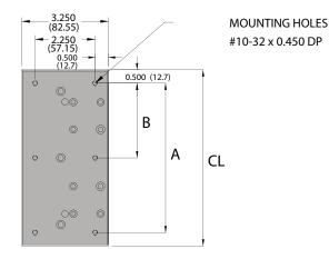
$$\begin{split} \text{TOTAL TRAVEL} &= \text{OAL - } 3.00" - \text{CARRIAGE LENGTH} \\ &= \text{OAL - } 76.2 \text{ mm} - \text{CARRIAGE LENGTH} \\ \text{OAL} &= \text{MULTIPLE OF 2.400" (} 60.96\text{)} \end{split}$$
