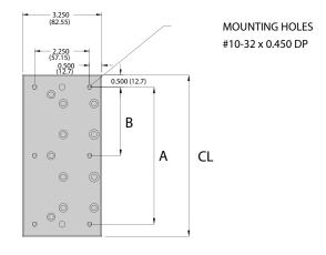
$$\label{eq:total_travel} \begin{split} \text{TOTAL TRAVEL} = \text{OAL - 3.00" } & (76.2) \text{ - CARRIAGE LENGTH} \\ \text{OAL} = \text{MULTIPLE OF 2.400" } & (60.96) \end{split}$$
