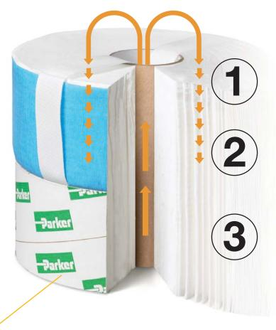
A card sleeve compresses the lower part of the element to increase the density and a non-woven cloth protects the base and stops particle migration.
