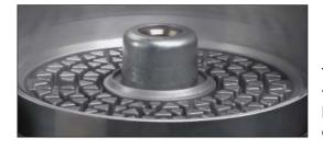
The intricately channeled base provides a large footprint to fully support the element under pressure, ensuring uniform loading of the element. Ultra-clean oil flows through the channels into the clean oil stream.
