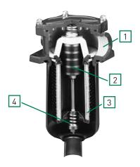
BGT Filters feature Parker's exclusive Magnetic Prefiltration core which collects ferromagnetic particles from fluid upstream of the filter element. This feature alone could save hundreds of dollars a year by protecting costly equipment from increased wear and malfunction by assuring that the fluid is as pure as possible when it leaves the filter. Even during bypass due to cold start up, ferris contaminant is collected by the magnetic core, a feature of importance on any fluid power system.
