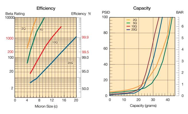
Results typical from Multi-pass tests run per test standard ISO 16889 @ 30 gpm to 100 psid terminal - 10 mg/L BUGL Refer to Appendix on pages 264-265 for relationship to test standard ISO 4572.
