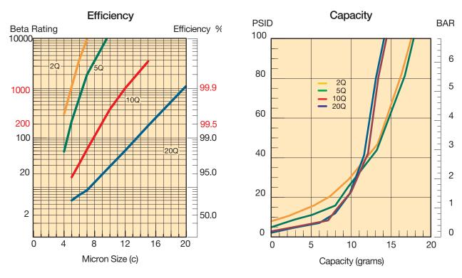
Results typical from Multi-pass tests run per test standard ISO 16889 @ 15 gpm to 100 psid terminal - 10 mg/L BUGL Refer to Appendix on pages 264-265 for relationship to test standard ISO 4572.
