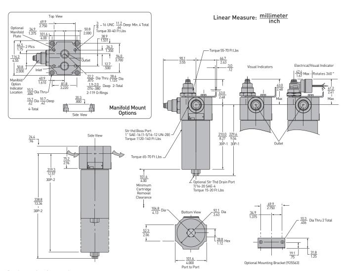
Drawings are for reference only. Contact factory for current version.
