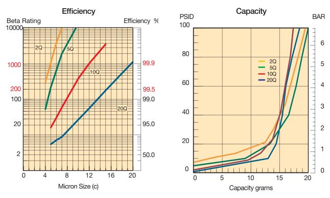
Results typical from Multi-pass tests run per test standard ISO 16889 @ 20 gpm to 100 psid terminal - 10 mg/L BUGL Refer to Appendix on pages 264-265 for relationship to test standard ISO 4572.
