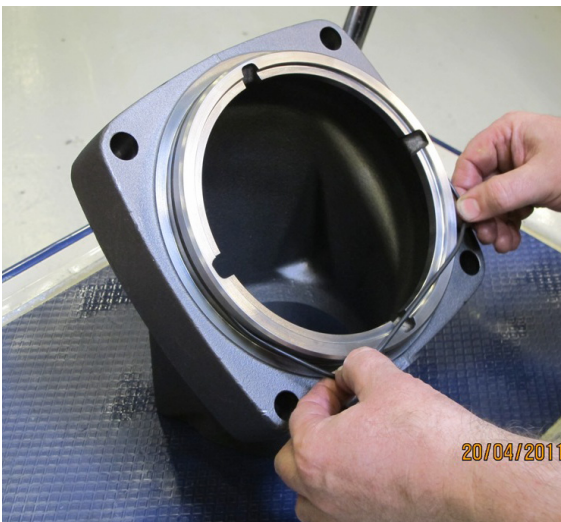
10. Assemble the O-ring (item 222) on the barrel housing (item 481). Lubricate the O-ring.
