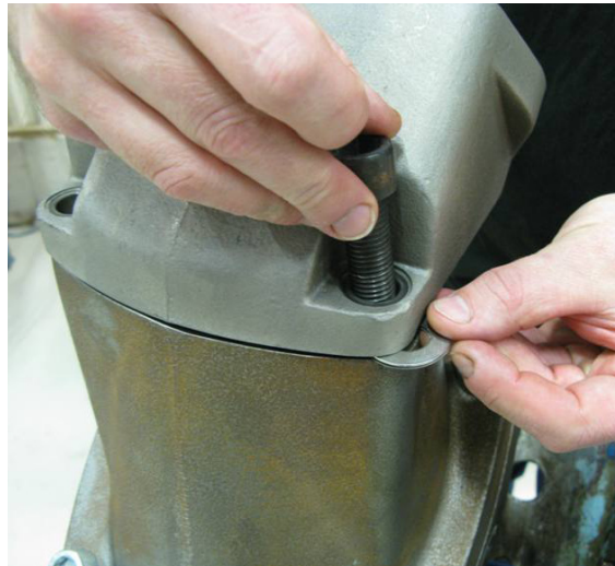
15. Knock down the end cap with a plastic hammer and fit shims (item 488) and hexagon screws (item 493). Torque the screws to 330 \pm 10 Nm.
