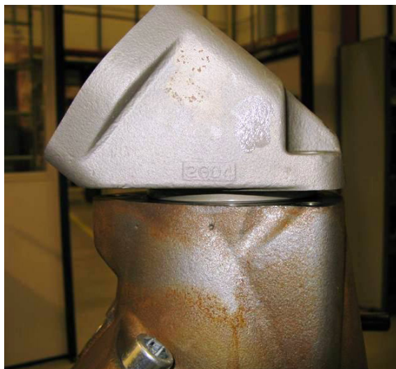
13. Place the end cap on to the barrel housing until the O-ring is entered.
