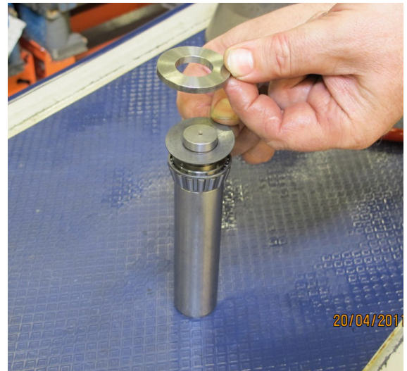
7. Assemble the tap roller bearing (item 425), the disc spring (item 433), the spacer washer (item 426) and the retaining ring (item 427).
