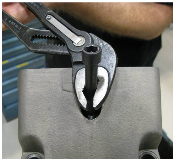
14. Fit a long screw (M12) to the barrel spindle and pull the barrel spindle up with a universal pliers.
