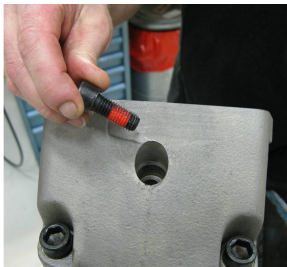
16. Install the cap screw (item 428) that secures the barrel spindle.
