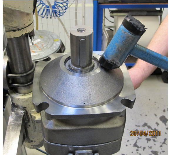
12. Assemble the bearing housing (item 211), tap it down with a plastic hammer. Torque the screws to 220 \pm 35 Nm.
