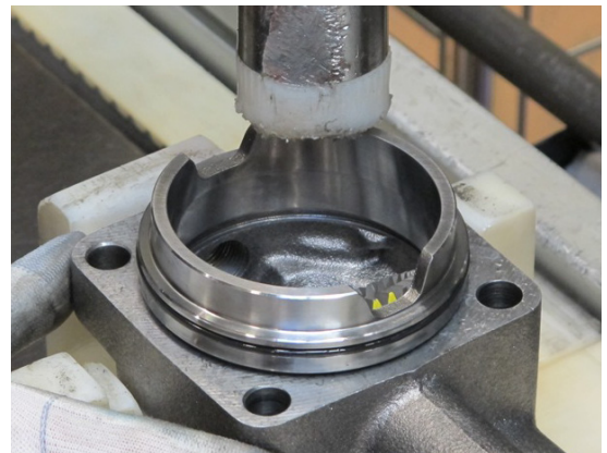
12. Carefully tap down the distance ring to the barrel housing. Lubricate them with oil before assembly.
