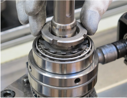
7. Assemble the round nut and tighten it until one opening is in correct position for the lock washer.
