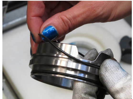
11. Assemble the O-rings on the distance ring.
