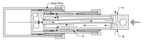
retracts in its turn, however, THE EFFECTIVE AREA FOR RETRACTING EACH STAGE IS THE AREA (D) OF THE PLUNGER.
