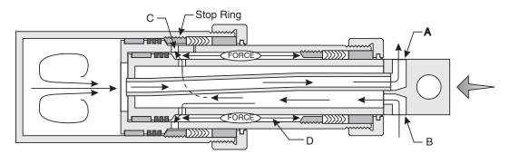
Oil inside the cylinder is forced out of port A. Because of the area differential, the flow into port B must be multiplied by this differential to determine the flow out of port A. It may be necessary to install a dump-to-tank valve to speed up the retracting cycle.
