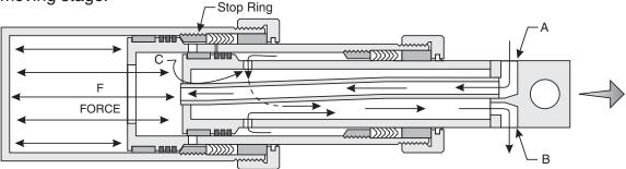
Oil trapped between the sleeves escapes through holes (C) in each sleeve and returns to the tank through port B.
