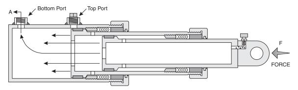
Under normal operating conditions the plunger or smallest diameter sleeve is pushed closed first, forcing oil out through port (A), then the next smallest, etc.
