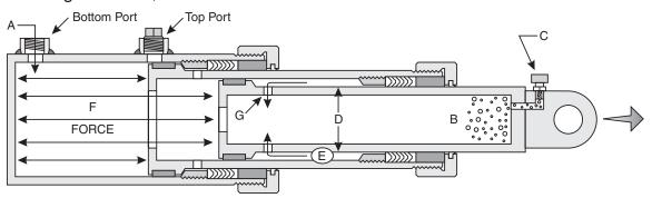
So at a given PSI (pressure) and GPM (gallons per min.) the cylinder will develop less force and increase in speed as it changes to the next moving stage.
