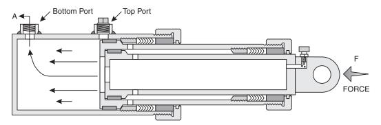
**Note:** If the top port is used, the speed of the cylinder may be reduced because of the oil flow restriction as the oil passes thru the transfer holes (G).
