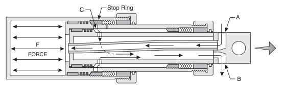
The effective area of each stage is figured from the inside diameter of the next largest stage. Each stage extends in its turn to the stop ring. So at a given PSI (pressure) and GPM (gallons per min.) the cylinder will develop less force and increase in speed as it changes to the next moving stage.
