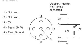
Pins are as seen on valve (male pin connectors)
