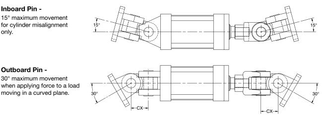
\*Maximum movement is achieved with cast clevis brackets. Movement is reduced when using fabricated clevis brackets.
