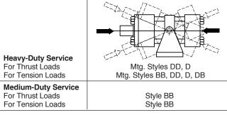
Group 3 FIXED MOUNTS which do not absorb force on the centerline
