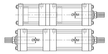
Reduced operating pressure is required for this construction. Please contact the factory.
