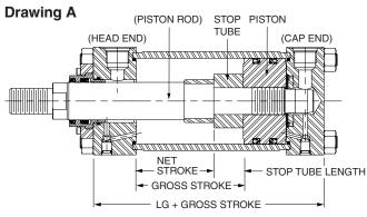
When specifying cylinders with long stroke and stop tube, be sure to call out the net stroke and the length of the stop tube. Machine design can be continued without delay by laying in a cylinder equivalent in length to the NET STROKE PLUS STOP TUBE LENGTH, which is referred to as GROSS STROKE.
