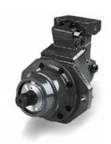
The T12 two-displacement motor is tailor-made for track drives. It allows a high ratio between high and low speed and installs as easily as a fixed displacement motor. Max speed ratio is 3.33-to-1. The T12 is a cartridge motor based on the well proven V12 series. The specially designed end cap with dual side ports permits a very short installation. A simple setting device moves the cylinder barrel to the maximum or
