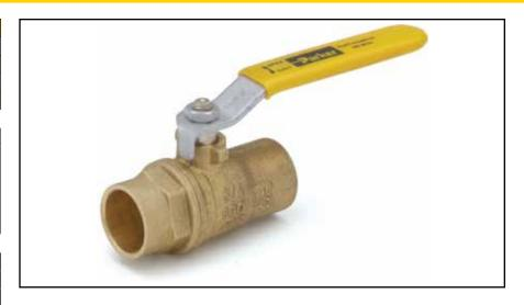
Parker's industrial ball valve product line is intended for general purpose use. Please be aware that ball valves are intended for use in the fully open or closed positions. Depending on application conditions, throttling of the valve may result in premature seal failure and/or inability to turn the valve handle.
