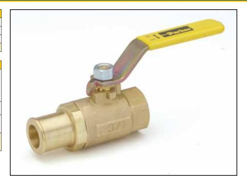
Parker's industrial ball valve product line is intended for general purpose use. Please be aware that ball valves are intended for use in the fully open or closed positions. Depending on application conditions, throttling of the valve may result in premature seal failure and/or inability to turn the valve handle. For use on construction equipment, chemical processing, plastic and rubber manufacturing, pumps, power units, and specialized industrial machinery requiring total shut-off capability.
