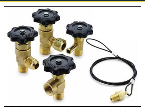
Truck valves have metal-to-metal seats with fine thread screwdown. The lanyard valves' compact design is ideally suited for releasing condensate from air tanks. Brass construction with specially formulated low temperature seal which remains elastic to temperature as low -40°F.
