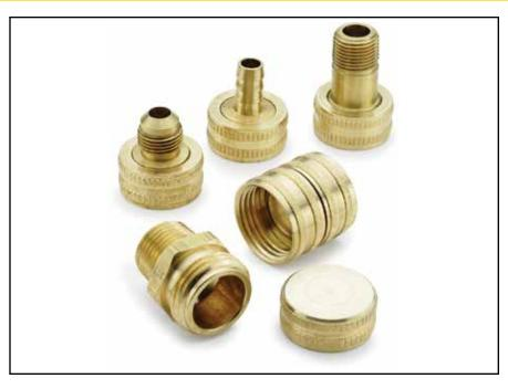
Connect garden hose to other garden hose, to pipe, or to tubing with these solid brass fittings. Hose-end threads are 3/4" garden hose thread. Swivel connectors allow hose to twist without kinking.
