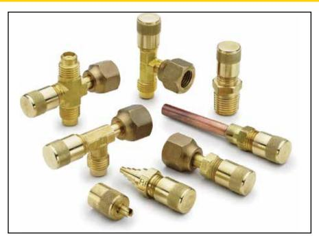
Designed to offer convenient low cost access ports for refrigeration service. All fittings feature 1/4" SAE male flare access ports and are furnished with a finger tight quick seal cap. Access valves with pipe connections have internal ODS solder cups.
