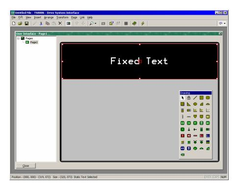
Only the US English text can be edited directly. The international versions of the text must be edited via the properties dialog box, which is accessed by selecting the object and pressing **Alt+Enter**, or by selecting the Properties command from the Edit menu.
