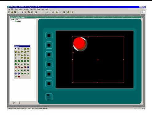
The now-reduced image can be moved within the whole object by defining values to control its horizontal and vertical position. These values are defined together with minimum and maximum limits that specify the values corresponding to the extremes of the image's movement within the object's bounding rectangle.
