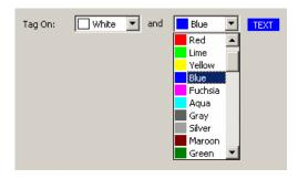
Color properties within the data tag represent a foreground and a background color that will be used to display the tag's state in textual form. Either of these colors can then be used to define the color of other animation objects. The example shows a color pair being edited. The drop-down list contains the sixteen standard VGA colors, the user-defined custom colors, and fourteen shades of gray.
