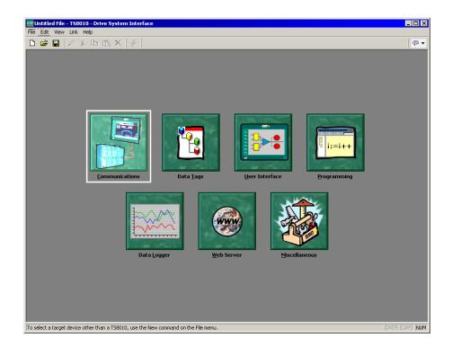
The software is designed such that the first three icons are the only ones required for the majority of simple applications. The remainder of the icons provide access to the terminal's more advanced features, such as programming, data logging and the unit's web server.
