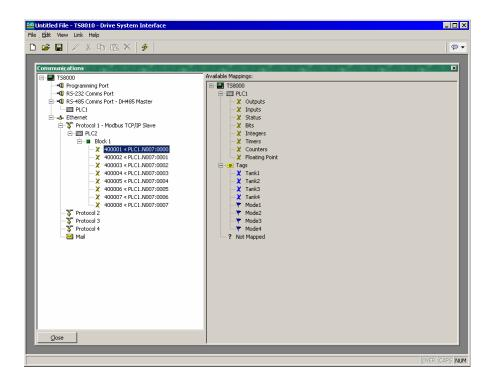
In this example, registers N7:0 through N7:7 in an Allen-Bradley controller have been exposed for access via Modbus TCP/IP as registers 40001 through 40008. DSI will automatically ensure that these data items are read from the Allen-Bradley PLC so as to fulfill Modbus requests, and will automatically convert writes to the Modbus registers into writes to the PLC. This mechanism allows even simple PLCs to be connected on an Ethernet network.
