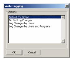
This indicates whether changes made to a tag by users or by programs should be logged. This facility allows you to create an audit trail of changes to your system, thereby simplifying fault finding and providing quality-control information as to process configuration. Note that care should be taken when logging changes made by programs, as certain database may log unmanageable amounts of data in such circumstances.
