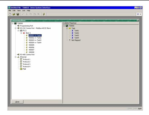
To indicate that you want a particular register within your gateway block to correspond to a certain data item, simply drag that item from the right-hand pane to the left-hand pane, dropping it on the appropriate gateway block entry. The example above shows how the registers **40001** through **40004** in the block above have been mapped to tags called **Tank1** through **Tank4**.
