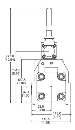
Note: 57mm (2.24") from bottom of bolt hole counterbore to bottom of valve.
