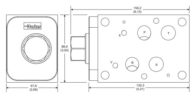
$\pmb{CH07TT} - \text{Inch equivalents for millimeter dimensions are shown in (**)}$
