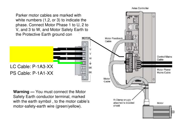
**Important** — An R-clamp must be connected to the drive and snugly attached to the exposed braided shield of the motor cable in order to control electrical noise.
