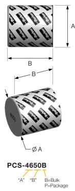
"A" and "B" dimensions in mm. Shorter length capsules recommended for elbow/bent fittings.
