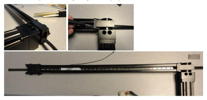
Wrap the belt around the drive and idler pulleys and bring belt ends to carriage. Make sure the tension plates are fixed as stated on previous page( pushed toward the base extrusion.). Lay Belt teeth on carriage teeth as shown. Make sure to achieve at least 5 teeth engament of belt on each side and then place/mount top of carriage to clamp belt utilizing the Qty2 socket head fasteners..
