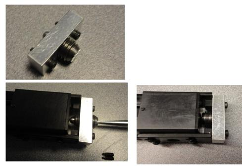
Now tighten the qty button heads that secure the tension plates into position. Remove the belt tension fixture Re-insert the flat head set screws.
