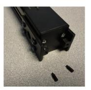
Remove the flat head set screws in the tension plates
