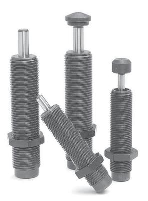
SC<sup>2</sup> 300 and SC<sup>2</sup> 650 Heavyweight Series Shock Absorbers deliver up to 950% of the effective weight capacity and 280% of the energy absorption capability of standard models. These durable units are ideal for decelerating heavy weights moving at low velocities. The Heavyweight Series design combines the piston and the inner tube into a single component, the piston tube. It acts as both the pressure creating and pressure controlling device.
