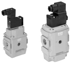
Parker Global Series Combined Soft Start / Dump Valves, provide for the safe introduction of pressure to machines or systems. Soft Start / Dump Valves when set, allow the pressure to gradually build to the set point before fully opening to deliver full flow at line pressure.
