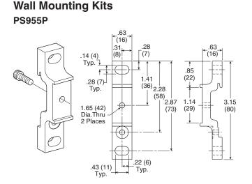
Wall Mounting Kits are available for mounting your Modular Assemblies and can be assembled and used with any standard body connector set.
