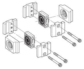
Port Block Connectors allow you to make threaded port connections to Modular units and are available in various port sizes to match your system requirements.
