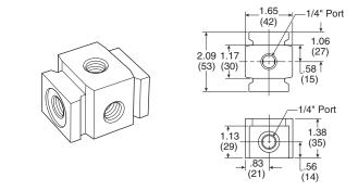
A Modular Manifold Block can be used between any two Modular units to give additional outlet ports. The 1/4" Manifold Block provides three additional outlets. Any standard pipe plug can be used to close off unused ports. **NOTE:** Body Connectors are not supplied with Manifold Blocks. Product Selection
