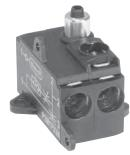
Depending on the application requirements, this vacuum generator may be controlled by single or by a dual 3/2 Moduflex valve. The Vacuum Generator has an integrated blow-off chamber that helps destroy the degree of vacuum. Blow-off can be increased with the addition of a control air input to the blow-off port on the vacuum module. A Ø6 mm port is available for an optional plug-in vacuum sensor for delivering a vacuum feedback signal.
