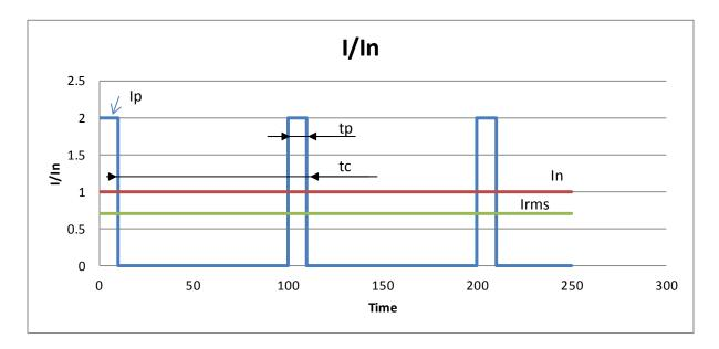
It is possible to use the GVM motors with a current higher than the permanent current (In). But, to avoid any overheating, the following rules must be respected.
