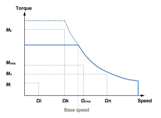
We are defining the base speed the knee of the continuous curve, not the knee of the peak curve...
