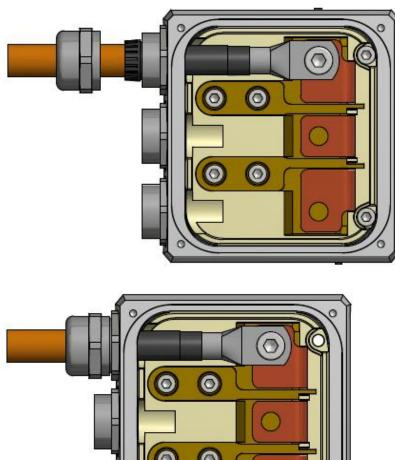
Please use M6 x 10 to fix the terminals (tightening torque : see p61)
